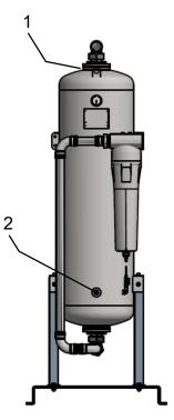
We recommend that you only change the filter element after the active carbon has been changed. To do so, allow the adsorber to run for half an hour. The dust particles that accumulate are hereby captured in the after-filter element which is to be replaced. Only then replace the filter element.
