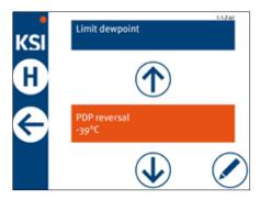
This value must always be higher than the TP trip value. It defines the value when the triggered alarm is automatically reset.
