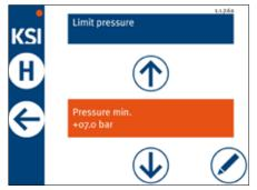
Set pressure for alarm triggering (incl. interruption function)
