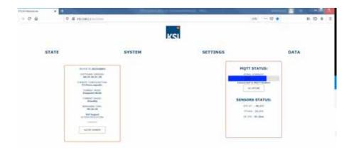
Normally you will be assigned the IPv4 address: 192.168.1.2 (from software version Ao.80 this is 192.168.1.124). You will only need this IP address in case of updates.
