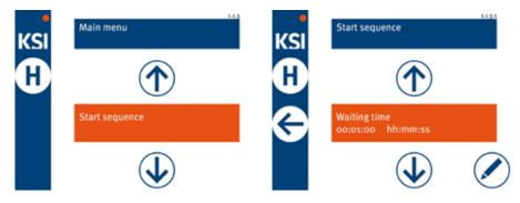
Here you can change the number of cycles and also define the time period until the first regeneration. This can be useful if, for example, you have carried out maintenance on the filter elements and the control should only run for a short cycle before returning to energy saving mode.
