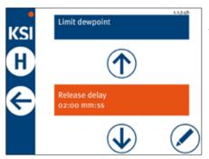
This time must be permanently below the TP trigger value for the alarm to become active.
