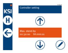
The stand-by time after reaching the set pressure dew point is defined here. The control now waits half an hour after reaching the pressure dew point before the next cycle is run. If the pressure dew point is exceeded again, regeneration starts immediately. The stand-by time can only be changed with a password.
