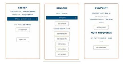
"Dewpoint" provides the possibility – if you are logged in – to set the control value (energy saving point) and also the forced switching time. You can also set the transmission frequency here under "MQTT Frequency" (IOT operation required for this). This should not be set for less than 60 seconds. Sensible frequencies for transmitting data extend the life of the IOT card.
