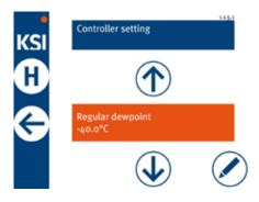
To set the pressure dew point for energy saving, please log in, press the pen and then enter the value. Afterwards the max. idle time will be set. This time defines how long the dryer will not regenerate as long as the pressure dew point is better than required.
